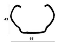
It is available in finishes available: Pre-galvanized steel Galvanized steel HOT COR-TEN
