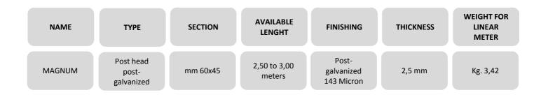
The pole is hot-dip galvanized after it is particularly suitable for areas near the sea.
