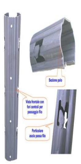
This pole is the pole ideal for vineyard mechanization high. The shape of the profile and the longitudinal ribs, combined with the quality and quantity (development of 135 mm) of the steel used, give our pole mechanical strength and flexibility, as well as a remarkable stability in the ground.
